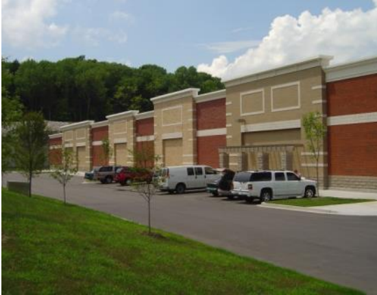
Figure 9-D: This figure shows two methods of using architectural features to create wall surface relief on wall elevations that are not the primary elevation.
