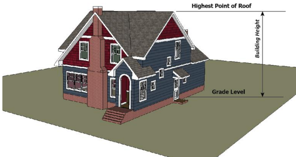
Figure 5-L: Measurement of building or structure height
