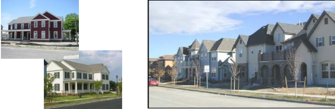
Figure 9-C: These images demonstrate how an attached residential structure of six or fewer units can be constructed to appear as a large detached residential structure.
